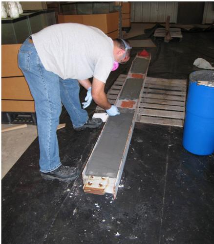
AMTS paste being applied to an I-beam contaminated with PCB paint
