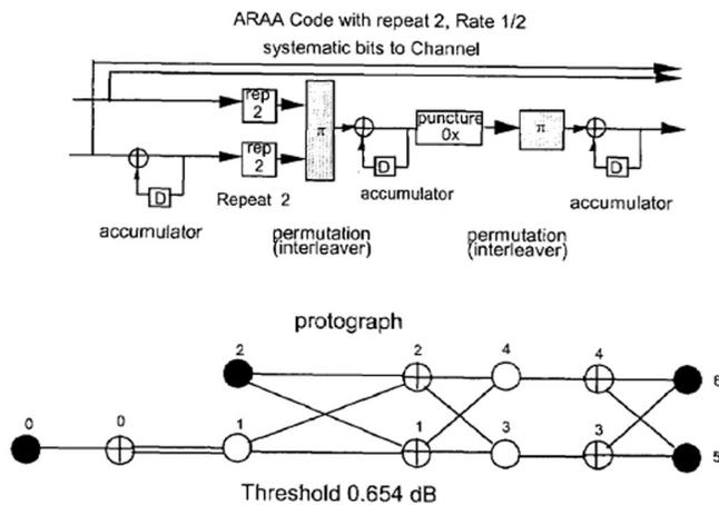
Accumulate-Repeat-Accumulate-Accumulate code. The concatenation of an accumulator as inner code with an ARA with repetition 2 as outer code provides a greater minimum distance than ARA codes and better suitability for low error floor applications.
