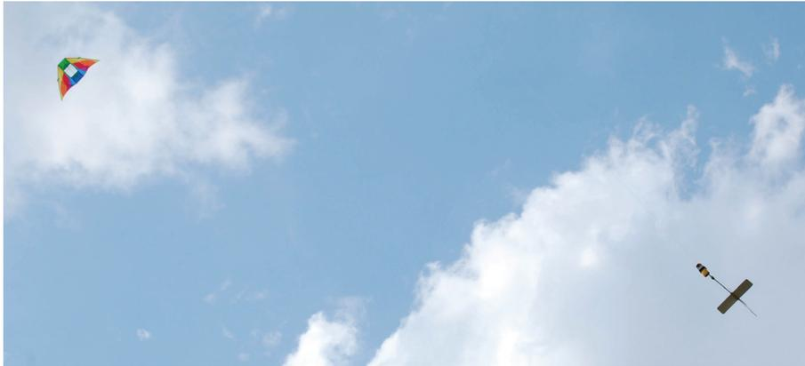
The Air Column Profiler Aeropod, being flown by a kite in the above photo, is used to capture a variety of atmospheric parameters throughout the air column.
