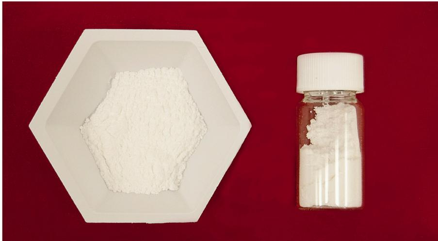
Flame suppression agent consisting of water droplets encapsulated in a flame retardant polymer
