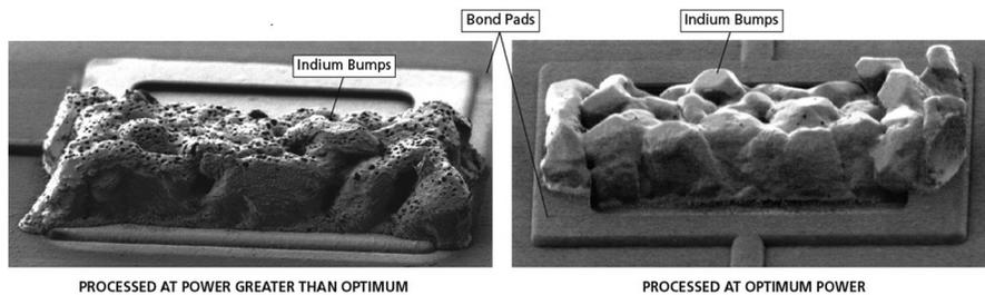
These Indium Bonding Bumps were treated by two different versions of the two-step plasma process. The pockmarks on the left bump were caused by greater-than-optimum plasma-generating power in the second step of the process. The right bump was processed at optimum power.
