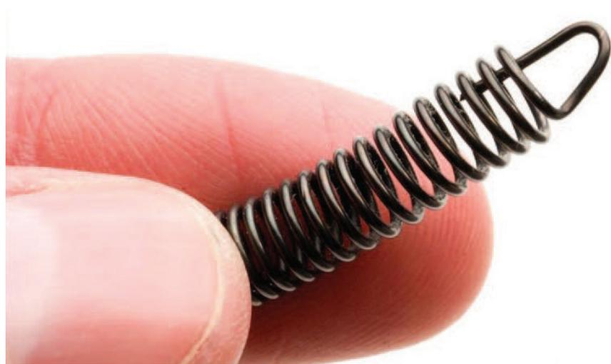
A spring made from a shape memory alloy.
