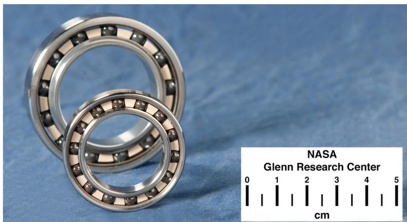
Bearings with NiTiNOL 60 balls and races
