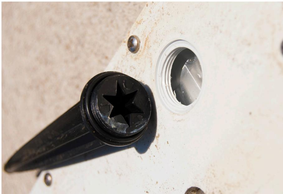
Star-shaped polymer spike removed from blanket reservoir
