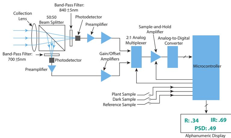
FIGURE – Schematic diagram of meter device, from original invention embodiment.
