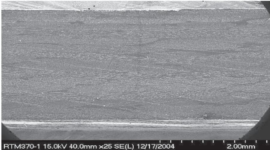
SEM cross section of a composite using RTM-370 as matrix material
