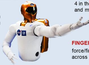
R2 can do all of these things side-by-side with humans. The robot moves at human speed. Its skin is soft and padded and it can sense through its safety systems when it comes into contact with someone. There are torsion springs inside the robot that provide force control – so when a person pushes away the robot's arm, it gives easily. And the robot always knows where its limbs are, making it safe for operation around people and delicate equipment.
