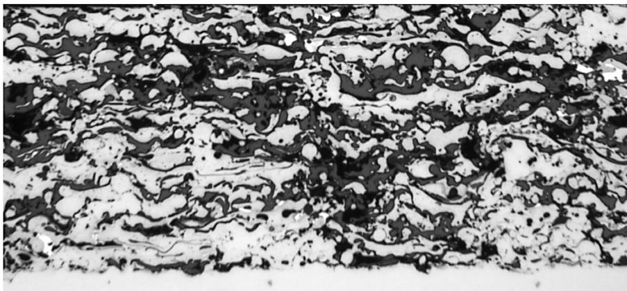
A PS400 cross-section control coating. The morphology is typical of plasma sprayed coatings and shows splat nature of constituent phases.
