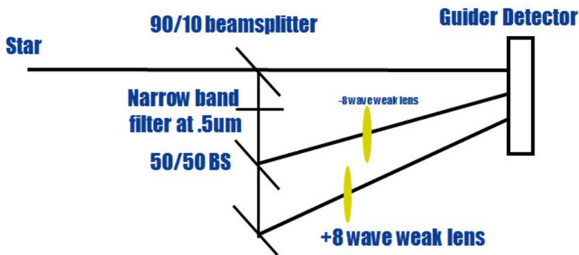
Schematic of the Hybrid Architecture Active Wavefront Sensing and Control system
